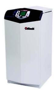
8 models, suitable for either Natural Gas or LPG - Advanced Control Systems − SMART SYSTEM™ Control - Cascade control for up to 8 Boilers - Fully modulating pre-mix burner - Outputs ranging from 41.2 to 228.4kW, based upon 50°C/30°C system design - Stainless steel heat exchanger - Weather compensation
