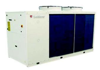
17 models with heating capacities of up to 210 kW - Suitable for LTHW and DHW applications - Low noise levels - Operates at up to 63°C water temperature - COP – up to 4.4 - Scroll compressors equipped with "Economised Vapour Injection - Interface card for Modbus control
