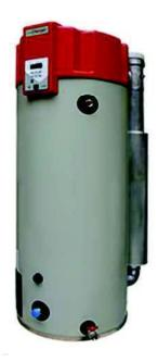
7 models, suitable for either Natural Gas or LPG - Fully modulating pre-mix burner - Multiple flue options - Recovery rates from 540 to 2100 litres/hour, based upon a 50°C temperature rise - Storage capacities from 220 to 488 litres - Ultra quiet operation - WRAS certified
